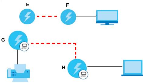
Figure 6 Two Separate Powerline Networks
