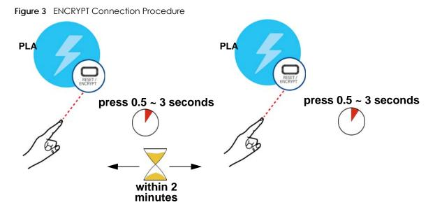
Note: The **RESET/ENCRYPT** button's location varies for each Powerline model.
